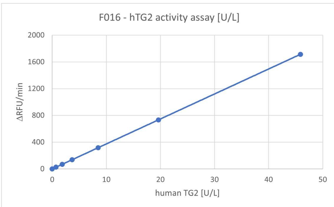
Figure 4: Enzyme Activity of a hTG2 REFERENCE in U/L, determined by dividing the increase of fluorescence ( $\Delta\text{RFU}/\text{min}$ ) by the extinction coefficient.
