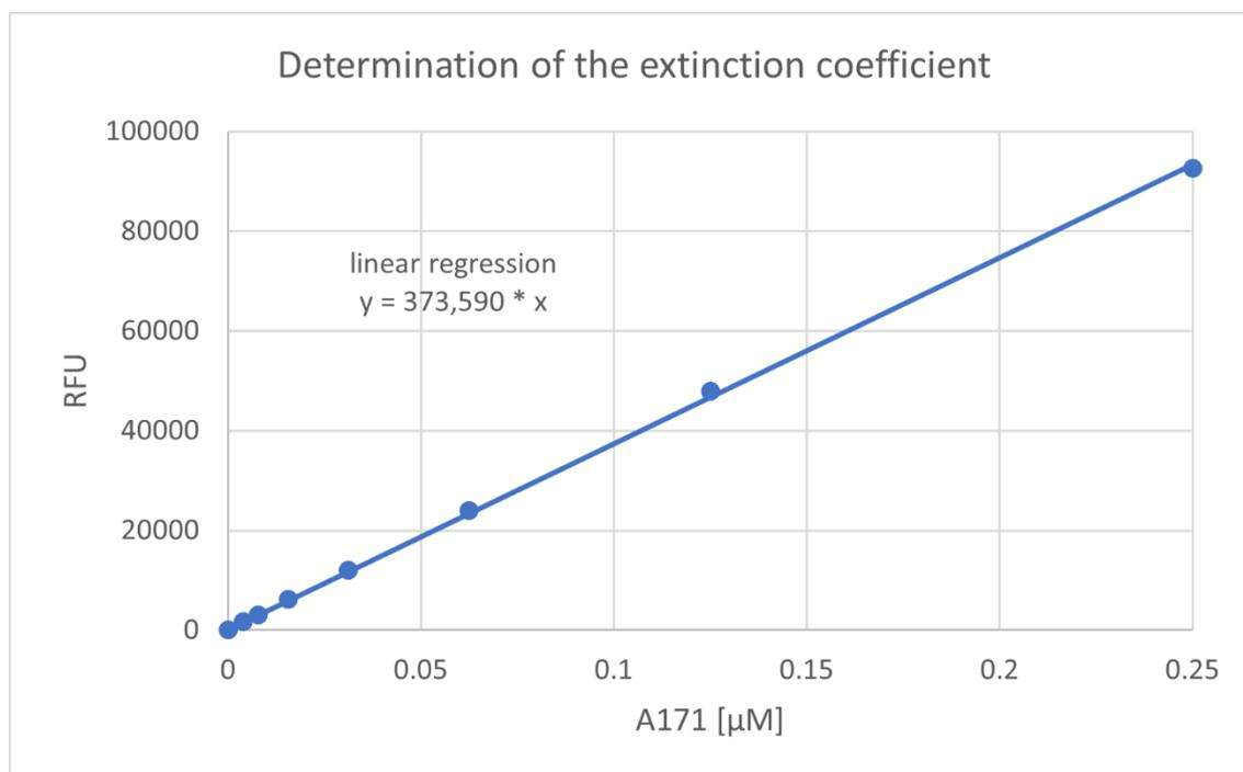
Figure 3: Determination of the extinction coefficient  $\epsilon$  [ $\mu\text{M}$ ]<sup>300 $\mu\text{L}$</sup>  by plotting the fluorescence (RFU) of a serial dilution of A171 (“N-ME-ABZ-PEPTIDE-CALIBRATOR”). The extinction coefficient equals to the slope of the linear regression.
